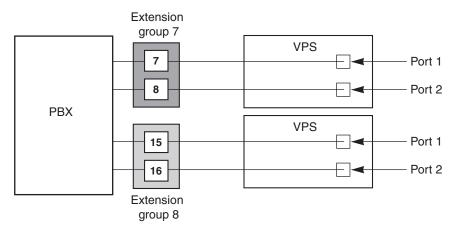
This example uses a Panasonic KX-TVS50 series VPS/KX-TVA50 series VPS, which can be connected with 4-conductor wire to 4 extension jacks of the PBX.
