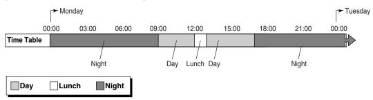
Note that time service modes can be arranged as they are needed (for example, night mode can occur in the morning and afternoon, if necessary) and not all time service modes need to be used in a time
